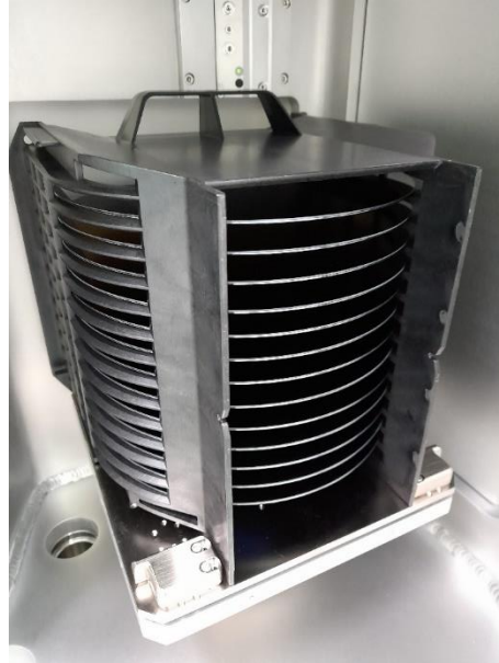
GaN-on-Si epiwafers from ALLOS Semiconductors, pictured in a cassette-to-cassette transfer module at ALLOS' manufacturing partner Ennostar
